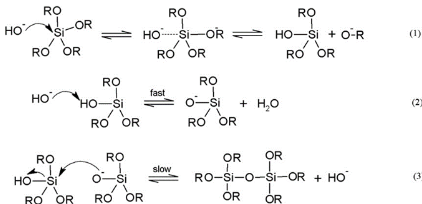
Fig. 1. Hydrolysis reaction (1) and Condensation reaction ((2) and (3)) of alkoxy silane in a basic catalyst
