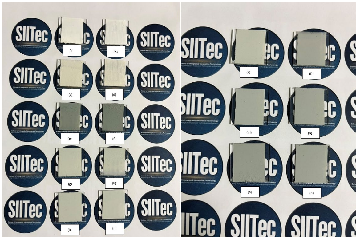
Fig. 1. Photographic images of nanocomposite films on glass substrates: (a, b) pure Roof Seal, (c, d) pure leucoxene, (e, f) pure CuS, (g, h) 1:9 composite, (i, j) 2:8 composite, (k, l) 3:7 composite, (m, n) 4:6 composite, and (o, p) 5:5 composite.
