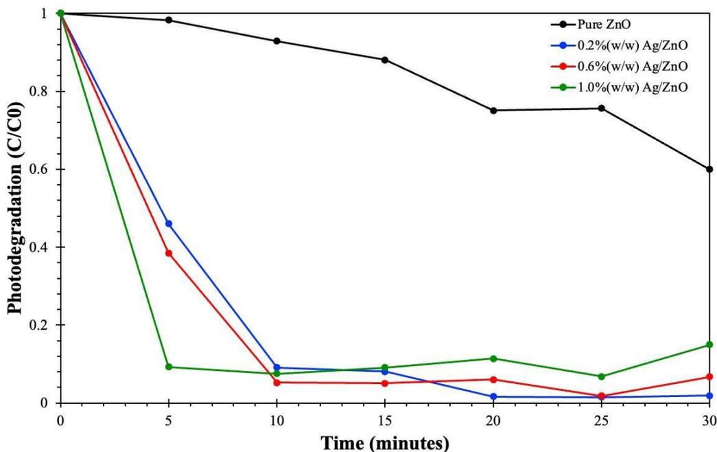
Fig. 5. Photodegradation of RhB solution under visible light irradiation using pristine ZnO and Ag NPs/ZnO composites with varying Ag loading levels.
