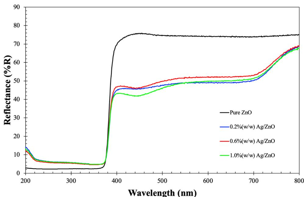
**Fig. 3.** Reflectance spectra of Ag NPs/ZnO composites with varying Ag loading contents.
