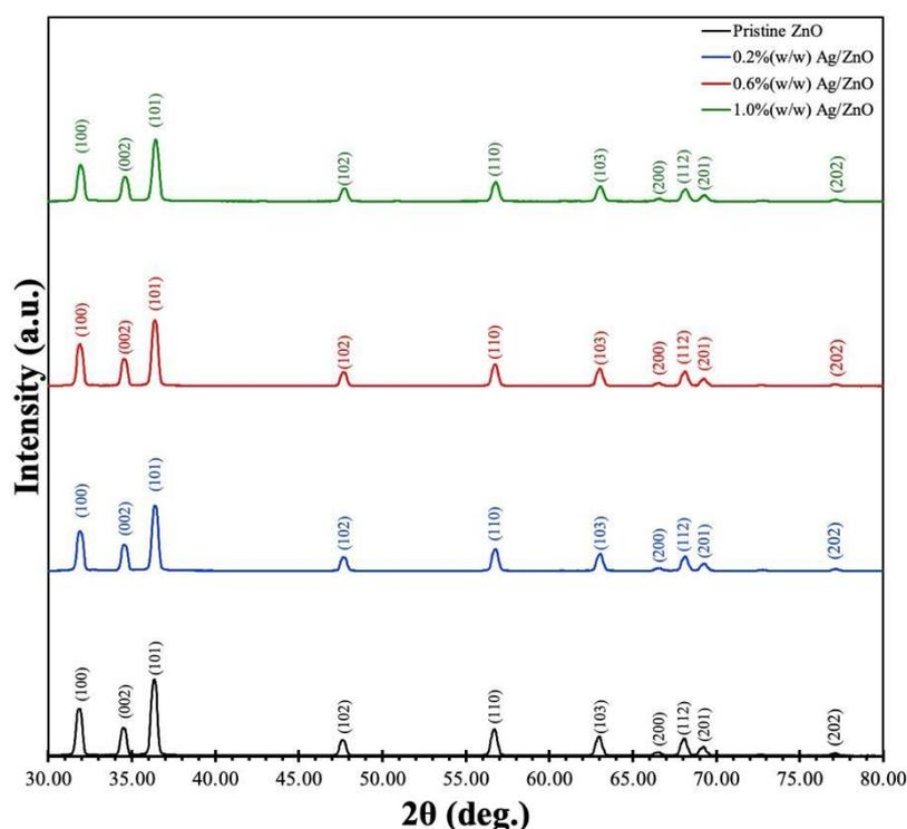
**Fig. 2.** X-ray diffraction patterns of Ag NPs/ZnO composites with varying Ag NP solution volumes: 0.2%, 0.6%, and 1.0%.
