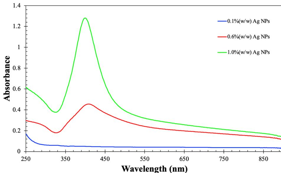
Fig. 4. Absorption spectra of Ag NPs with varying Ag loading contents.
