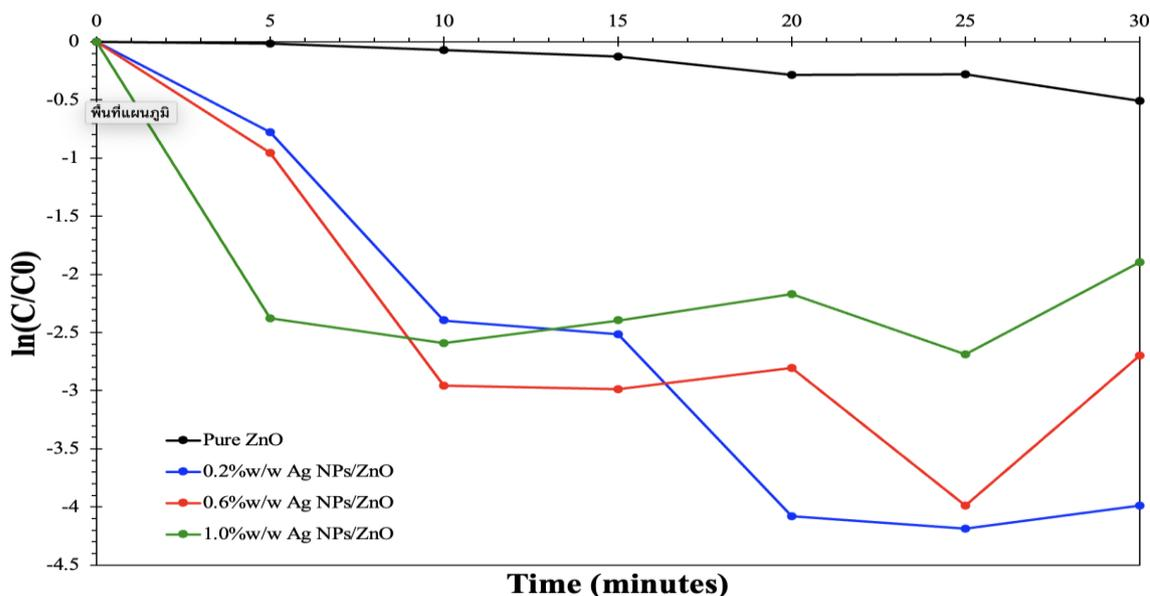
**Fig. 6.** Degradation rate of RhB for pristine ZnO and Ag NPs/ZnO composites under visible light irradiation at varying Ag loading contents.
