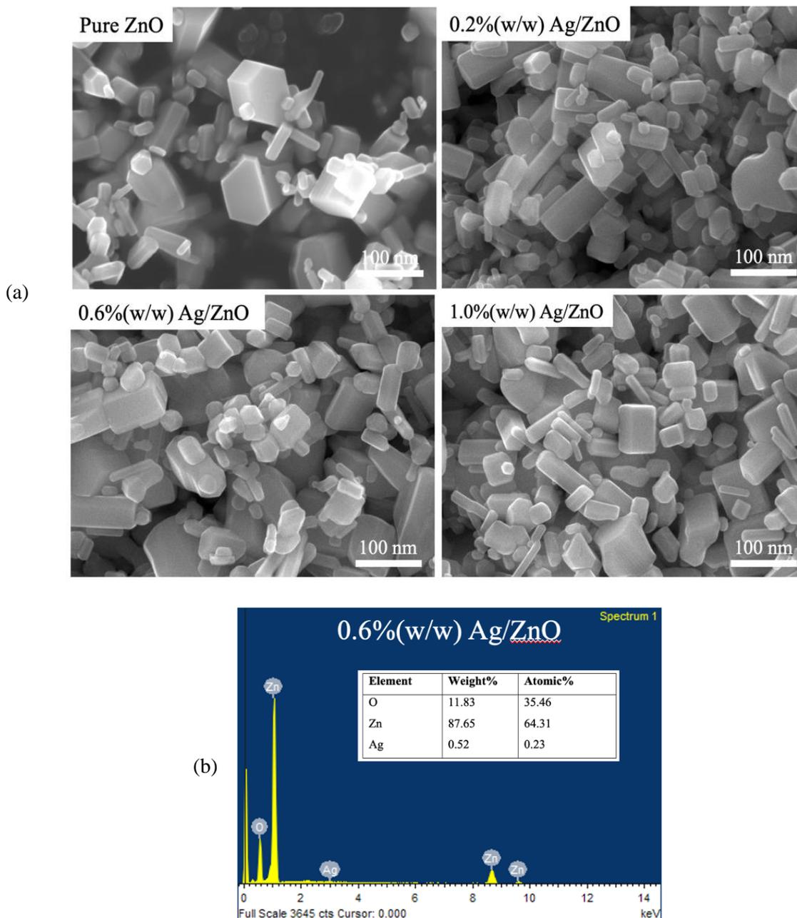
**Fig. 1.** (a) FE-SEM image of pristine ZnO and Ag NPs/ZnO composites showing the morphologies under various Ag NPs solution volumes. (b) EDX histogram of Ag NPs/ZnO composites displaying the elemental composition of the synthesized composites.
